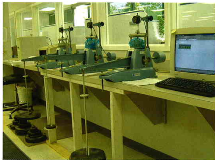
Consolidation Loading Device – Tests rate and magnitude of soil consolidation
